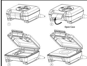
Plug audio jack into the shuffle player, place shuffle into case and ensure the control pad and the Button Pad Control are aligned. Close case.
